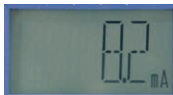
On screen commissioning aids include input signal, software travel switch status and valve diagnostics
