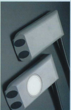
Figure 3: The MACE combined depth/velocity sensor on the right of the picture.
